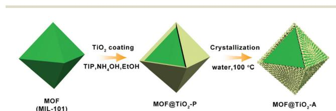
**Scheme 1** Schematic representation of the preparation of MOF@ $\text{TiO}_2$ -A core-shell nanostructures. Step 1: coating the MOF nanocrystal with an amorphous  $\text{TiO}_2$  shell to obtain MOF@ $\text{TiO}_2$ -P at room temperature. Step 2: water-assisted crystallization of MOF@ $\text{TiO}_2$ -P at 100 °C to obtain the well-crystallized MOF@ $\text{TiO}_2$ -A.
