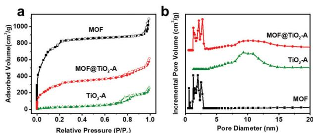
Fig. 4 Nitrogen adsorption–desorption isotherms (a) and pore size distribution curves (b) of MOF, TiO<sub>2</sub>-A and MOF@TiO<sub>2</sub>-A.
