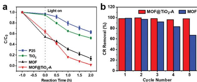
Fig. 5 Kinetic traces for CR adsorption and photodegradation in the presence of P25, TiO<sub>2</sub>, MOF and MOF@TiO<sub>2</sub>-A (a), and photodegradation stability of recycled MOF and MOF@TiO<sub>2</sub>-A (b).
