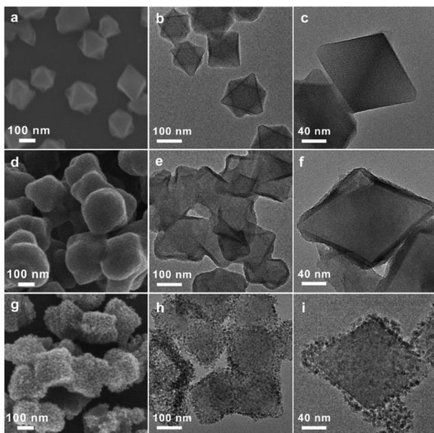
**Fig. 1** Morphological changes from MOF to MOF@TiO<sub>2</sub>-P and finally to MOF@TiO<sub>2</sub>-A core-shell nanostructures. SEM and TEM images of MOF (a–c), MOF@TiO<sub>2</sub>-P (d–f), and MOF@TiO<sub>2</sub>-A (g–i).
