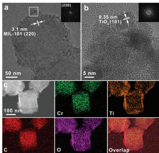
**Fig. 2** TEM images of a single MOF@TiO<sub>2</sub>-A core-shell nanoparticle (a) and enlarged high-resolution TEM image of the TiO<sub>2</sub> shell corresponding to the rectangular area in a (b). High-magnification HAADF-STEM image of MOF@TiO<sub>2</sub>-A (c) and the corresponding EDX elemental mapping results. Insets in a and b correspond to the fast Fourier transform (FFT) images of MOF and TiO<sub>2</sub> crystals.
