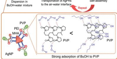
Scheme 1 Suggested mechanism for AgPR assembly at the air-liquid interface.
