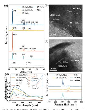
Fig. 3 (a) XRD pattern of HV-SnS<sub>2</sub>/MoS<sub>2</sub>, LV-SnS<sub>2</sub>/MoS<sub>2</sub>, HV-SnS<sub>2</sub>, LV- $SnS_2$ , and  $MoS_2$ . (b) TEM image of HV- $SnS_2/MoS_2$ . (c) TEM image of LV-SnS<sub>2</sub>/MoS<sub>2</sub>. (d) UV-Vis absorption spectroscopy of all samples. The inset is Tauc plot for estimating the bandgap energies ( $E_{q}$ ) of MoS<sub>2</sub> and HV-SnS<sub>2</sub>. (e) Raman spectra of all samples.
