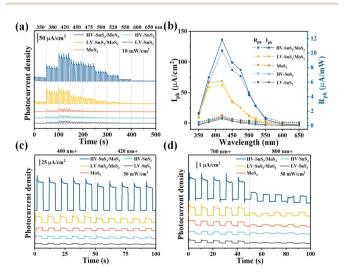
Fig. 6 (a) The amperometric l-t curves irradiated by light at different wavelengths. (b)  $I_{\rm ph}$  and  $R_{\rm ph}$  as a function of wavelength. (c) The amperometric I-t curves irradiated by light in 400+ and 420+ nm. (d) The amperometric I-t curves irradiated by light in 700+ and 800+ nm.
