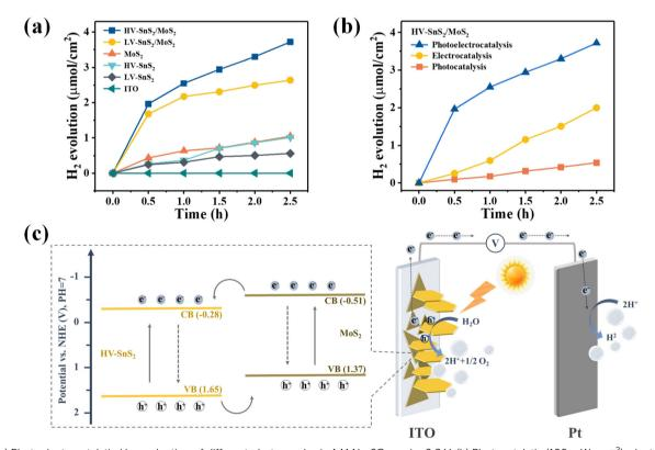
Fig. 9 (a) Photoelectrocatalytic  $H_2$  production of different photoanodes in 1 M  $H_2SO_4$  under 0.8 V. (b) Photocatalytic (100 mW cm $^{-2}$ ), electrocatalytic (0.8 V), and photoelectrocatalytic (100 mW cm $^{-2}$ , 0.8 V)  $H_2$  production of HV-SnS $_2/MoS_2$  photoanode. (c) The schematic plot of charge transfer pathways in HV-SnS $_2/MoS_2$  heterostructure as an effective photoelectrode for PEC water splitting.
