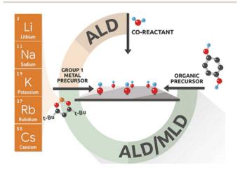
Fig. 4 Mechanism diagram of the atomic layer deposition (ALD) technique. Reproduced with permission from ref. 58, Copyright® 2021, American Chemical Society.
