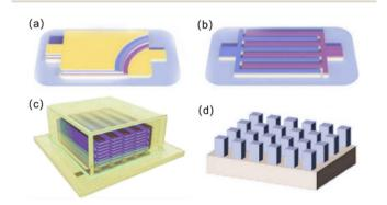
Fig. 2 Schematic diagrams of various micro-LIBs according to different cell microstructures: (a) laminated thin film structure, (b) planar interdigital structure, (c) 3D interdigital structure, (d) other types of 3D architecture (microtube structure).
