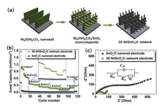
Fig. 11 (a) Fabrication process, (b) rate performance and (c) EIS plot of the 3D Ni/SnO $_x$ /C electrode. Reproduced with permission from ref. 81, Copyright© 2013, American Chemical Society.
