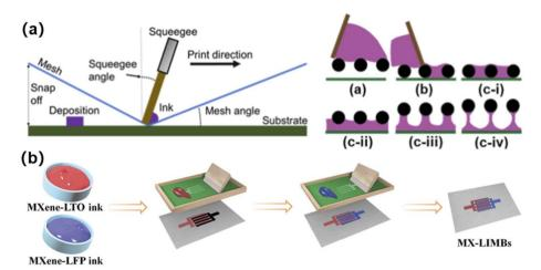
Fig. 7 (a) Schematic diagram of screen printing. Reproduced with permission from ref. 66, Copyright© 2021, American Chemical Society. (b) A screen printed interdigital micro-LIB prepared by using MXene-based electrode inks. Reproduced with permission from ref. 67, Copyright® 2021, Wiley & Sons.
