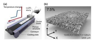
Fig. 5 (a) Schematic diagram of the tape-casting technique. (b) Porous  $\text{Li}_7\text{La}_3\text{Zr}_2\text{O}_{12}$  solid electrolyte prepared by tape-casting. Reproduced with permission from ref. 60, Copyright© 2020, American Chemical Society.
