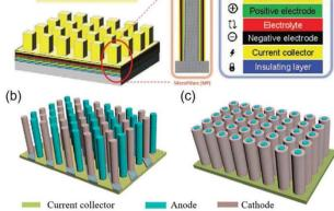
Fig. 3 Schematic diagrams of various micro-LIBs based on 3D microstructures: (a) 3D microtube structure. Reproduced with permission from ref. 49, Copyright@ 2017, Wiley-VCH Verlag. (b) 3D interlaced pillar structure and (c) 3D coaxial structure.
