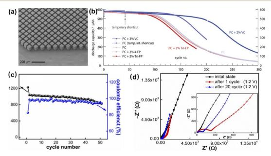
Fig. 12 (a) The anode compartment of a microbattery based on monocrystalline Si, and (b) cycling tests of the microbattery made of monocrystalline Si in different electrolytes. Reproduced with permission from ref. 85, Copyright© 2021, by the authors. (c) Cycling performance and (d) EIS plots of a Sn-Si anode. Reproduced with permission from ref. 86, Copyright© 2021, by the authors.
