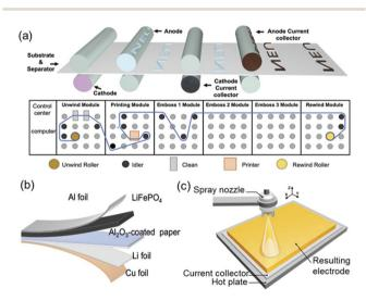
Fig. 6 (a) Schematic diagram of flexographic printing and (b) a thin-film lithium metal battery based on the flexographic printed LiFePO<sub>4</sub> cathode. Reproduced with permission from ref. 62, Copyright© 2022, Wiley-Blackwell. (c) Schematic diagram of spray printing for preparing thin film electrodes of LIBs. Reproduced with permission from ref. 63, Copyright© 2018, Elsevier Ltd.
