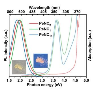
Fig. 3 UV-Vis absorption and PL spectra of PeNC $_0$  ( $\lambda_{ex}=275$  nm), PeNC $_1$  ( $\lambda_{ex}=330$  nm), and PeNC $_1$ 0 ( $\lambda_{ex}=330$  nm) with nanocrystals in the powder form. Photographs showing the PeNC $_1$  powder sample under room illumination (left) and UV irradiation (right).
