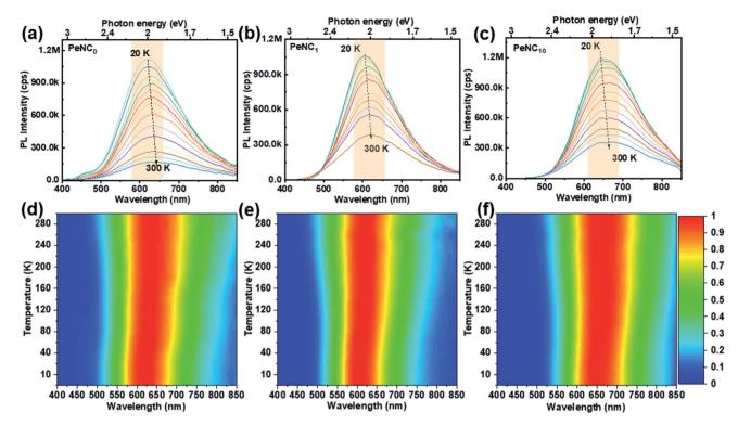
Fig. 4 Temperature-dependent PL spectra of (a)  $PeNC_0$  ( $\lambda_{ex} = 275 \text{ nm}$ ), (b)  $PeNC_1$  ( $\lambda_{ex} = 330 \text{ nm}$ ), and (c)  $PeNC_{10}$  ( $\lambda_{ex} = 330 \text{ nm}$ ) from 20 to 300 K. Normalized PL intensity mapped with the emission wavelength and temperature for (d)  $PeNC_0$  (e)  $PeNC_1$ , and (f)  $PeNC_{10}$ .
