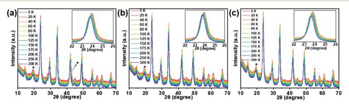
Fig. 2 LT-XRD patterns of (a) PeNC<sub>1</sub>, (b) PeNC<sub>1</sub>, and (c) PeNC<sub>10</sub> in the temperature range from 5–300 K. Peaks indicated as  $\star$  and  $\bullet$  are from the X-ray window materials of the cryostat and from the Cu sample holder, respectively.
