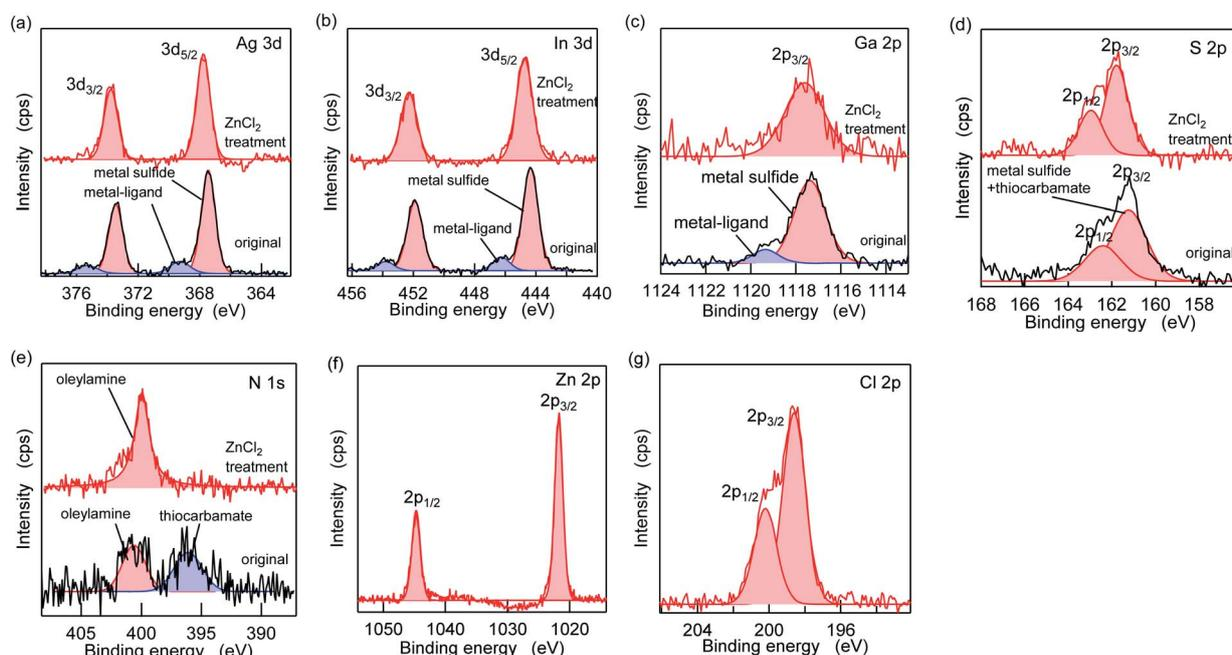
Fig. 5 XPS spectra of the pristine AIGS QDs (black lines) and the ZnCl<sub>2</sub>-treated AIGS QDs (red lines). (a) Ag 3d, (b) In 3d, (c) Ga 2p, (d) S 2p, (e) N 1s, (f) Zn 2p, and (g) Cl 2p. (f) and (g) display the treated samples only.
