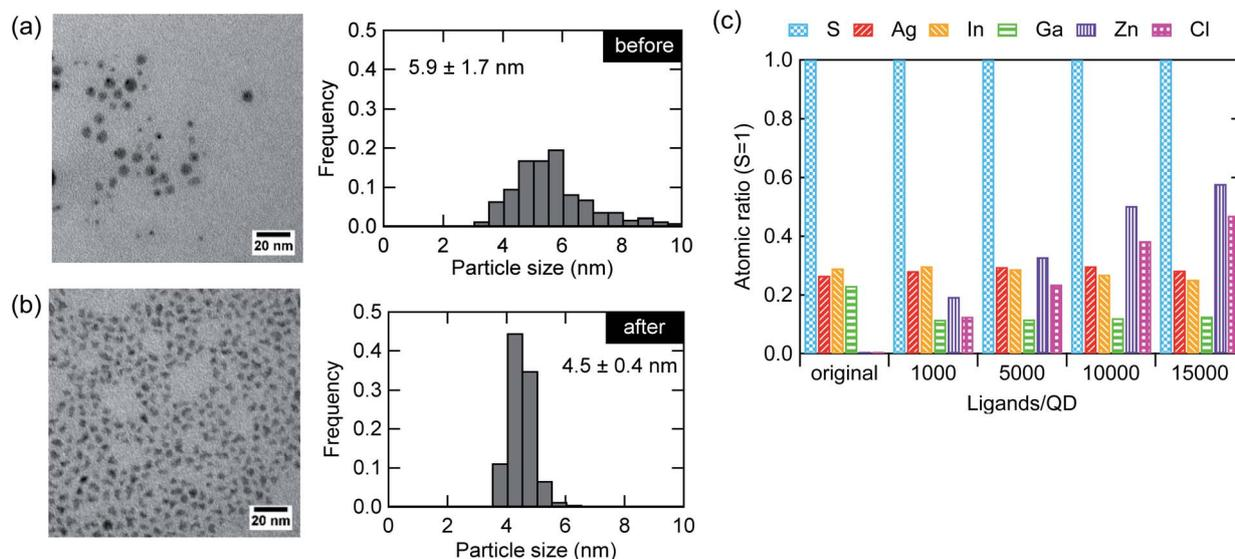
Fig. 4 TEM images and corresponding size distribution histogram of the AIGS QDs (a) before and (b) after  $\text{ZnCl}_2$  addition at mole ratio of 10 000 ligands/QD. (c) Atomic ratio (sulfur basis) of the original AIGS QDs and the QDs after  $\text{ZnCl}_2$  addition at mole ratios in the range of 1000–15 000 ligands/QD.
