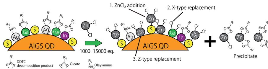
**Scheme 1** Schematic of the proposed mechanism of ligand exchange; (process 1) the addition of  $\text{ZnCl}_2$ , (process 2) replacement of the X-type ligands, and (process 3) replacement of the Z-type ligands.
