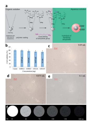
Fig. 1 Organic functional group modification of FePt-CdS NPs. (a) Schematic showing the preparation process of water-soluble FePt NPs and FePt-CdS NPs. (b) Cell compatibility test. Addition of different concentrations of (c) 0.05 mL (d) 0.075 mL and (e) 0.1 mL polymeric FePt NPs. (f) MRI contrast analysis at different FePt NP concentrations. This figure has been reproduced from ref. 50 and 51 with permission from ACS Publications and Elsevier, copyright 2017 and 2019.
