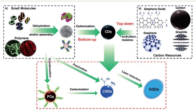
Fig. 3 Schematic illustration of the production routes of CDs: (a) "bottom-up" synthesis, where CDs are prepared from organic molecules or polymers through hydrothermal, calcination, microwave radiation, and not limited to these methods; (b) "top-down" synthesis, where CDs are prepared from larger sized carbon resources through acidic oxidation, hydrothermal cutting, and electrochemical methods.
