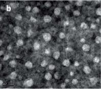
Fig. 8 The scheme depicts the preparation of a gene delivery platform using CDs as vehicles. (a) The CDs are prepared through microwaveinduced hydrothermal treatment of glycerol and polyethyleneimine. The CDs were incubated with DNA, forming the transfection agent following further condensation; (b) TEM images of negatively stained CDs/pDNA complexes. They were adopted and modified from. 76 These images were adapted with permission from ref. 76. Elsevier, copyright 2021.
