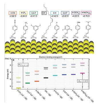
(Top) The molecular structures of organic molecules on PbS QDs and their dipole intensity; (bottom) the shifting of energy levels from the surface treatments with the dipole molecules determined by UPS. Reproduced with permission from ref. 31
