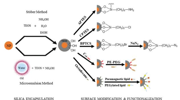
Fig. 4 Silica encapsulation of nanoparticles (orange) can be achieved by two main methods: the Stöber method and the microemulsion method. The surface of the silica shell is rich in hydroxyl groups, which can be modified and functionalized by silane coupling agents, polymers, or lipids. APTES = (3-Aminopropyl)triethoxysilane; CPTES = (3-Chloropropyl)triethoxysilane; BPTCS = (3-Bromopropyl)trichlorosilane.
