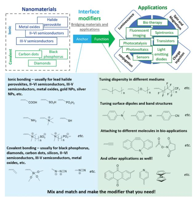
Fig. 1 An interface modifier can be seen as molecule comprised of two key components: (i) anchor groups that attaches to inorganic nanomaterials, and (ii) functional groups that tune the properties of inorganic nanomaterials to better suit the target applications. Some examples of anchors and functional groups are shown here
