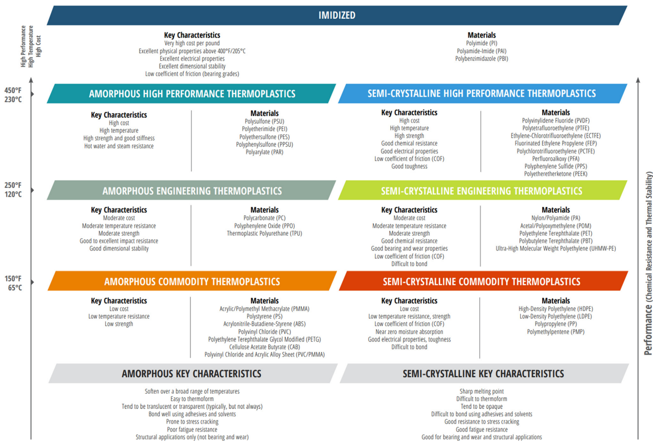
Fig. 6 International Association of Plastics Distribution Thermoplastics Rectangle. Reproduced from ref. 34 with permission from International Association of Plastics Distribution, copyright 2021.
