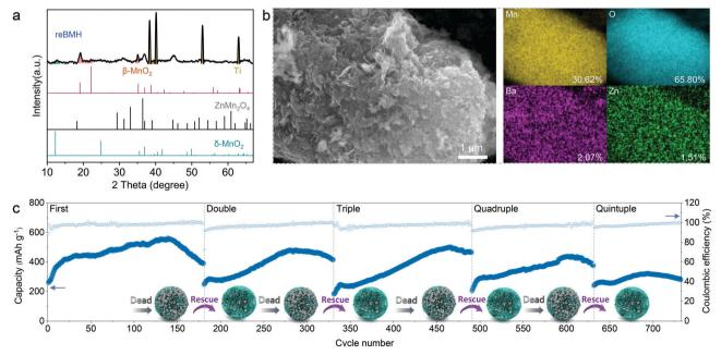
Fig. 5 Rescue of the dead BMH electrode. (a) XRD pattern of the reBMH electrode. (b) SEM/EDX images of the reBMH electrode. (c) Electrochemical performance of reBMH at a current density of 0.3 A g<sup>-1</sup> with the rescue for 5 recycles.
