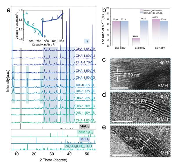
Fig. 2 Charge storage mechanism. (a) Ex situ XRD patterns of the BMH cathode in selected states in the 2nd discharge/charge cycle. (b) Analysis of reversible change in the ratio of Mn<sup>4+</sup> at different states by XPS spectra in different electrolytes. (c-e) TEM images of three samples at the fully charged state of 1.85 V. Scale bar, 5 nm
