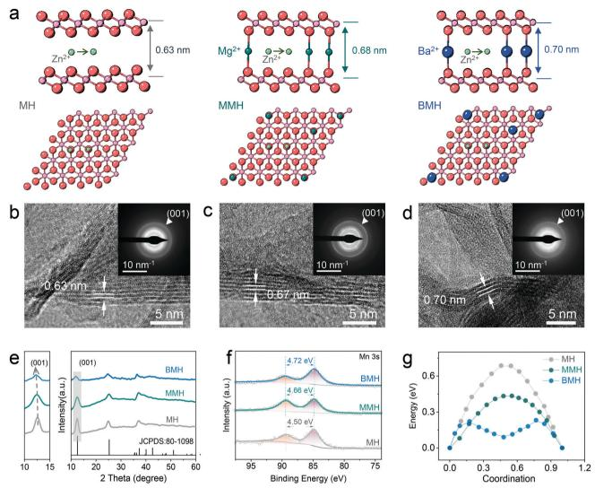
Fig. 1 Design and characterization of MH, MMH, and BMH. (a) Calculation model and possible migration path of Zn<sup>2+</sup>. (b-d) TEM images, (e) XRD patterns, and (f) XPS spectra of Mn 2p. (g)  ${\rm Zn^{2+}}$  migration energy in different materials
