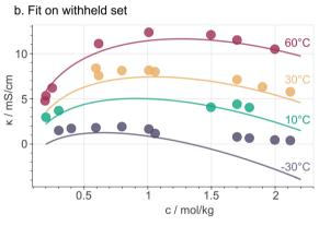
Fig. 3 (a) Root mean square error of selected model (green) and benchmarks (red) on the validation set, compared to measurement dispersion (grey). (b) Fit of the selected model on the withheld (validation and test) set at r=1.0.
