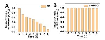
Fig. 4 Variations in the absorption intensity ratio at 450 nm of BP (A) and BP/Bi<sub>2</sub>O<sub>3</sub> heterostructures (B) after standing in water for different durations of time. Adapted and modified with permission from ref. 26 Copyright (2018) Elsevier.
