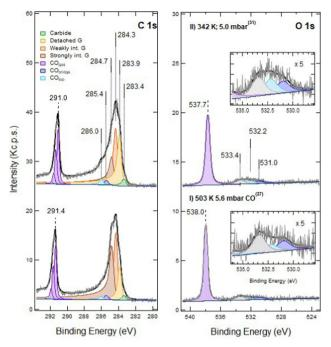
Fig. 4 NAP-XPS spectra of the C 1s (left) and O 1s (right) regions for sputtered G/Ni(111) (60 s at RT; ion energy of 150 eV) during CO exposure: (I) at 503 K and  $P_{CO}$  = 5.6 mbar; (II) after cooling down to 342 K and  $P_{\text{CO}}$  = 5.0 mbar. The spectra are plotted in absolute counts since the data were recorded in similar NAP conditions and at different sample temperatures so that no evident normalisation protocol can be applied.
