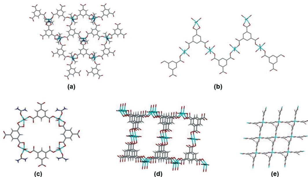
Fig. 8 Motifs observed for simple  $btc$  coordination polymers. (a) Hexagonal network, illustrated by ADOLUB,<sup>48</sup> (b) 2D tape, illustrated by TOPMIU,<sup>49</sup> (c) discrete quadrilateral motif, illustrated by OXAWOB,<sup>50</sup> (d) quadrilateral spiral network, illustrated by JEQNUP,<sup>51</sup> and (e) square-grid network, illustrated by MITRUD.<sup>52</sup>
