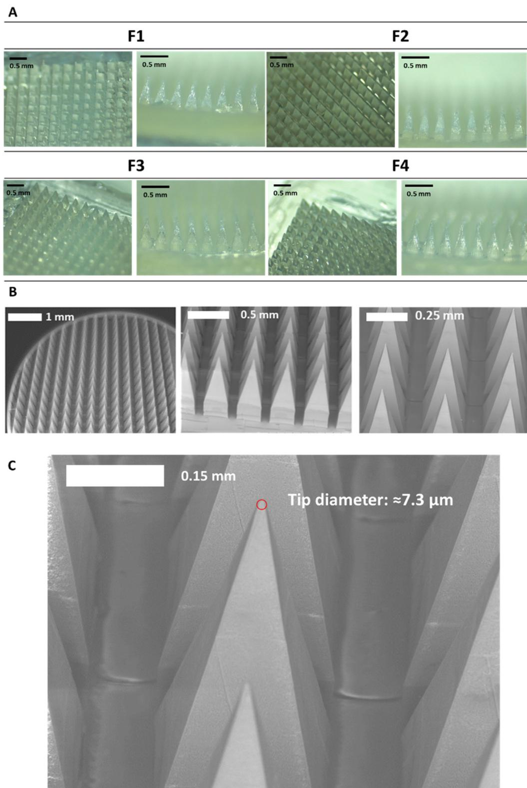
**Fig. 4** (A) Optical microscopy images of CLC-Soluplus® microarray patches (MAPS) with different Soluplus® concentration fabricated *via* double casting method. (B) SEM images of dissolving MAPs fabricated from Soluplus® which are loaded CLC. (C) Microneedle tip diameter of CLC-loaded MAPs,  $\approx 7.3 \mu\text{m}$  ( $n = 5$ ).
