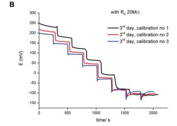
Fig. 4 (A) Selected potentiometric calibration plots for potassium-selective ISE, bypassed by zinc wire and resistor  $R_b = 20 \text{ M}\Omega$ , third calibration for each consecutive day is presented: (**II**) 1st day, (**II**) 2nd day ( $\bigcirc$ ) 3rd day. (B) Time traces for the sequential calibrations of the 3rd day.
