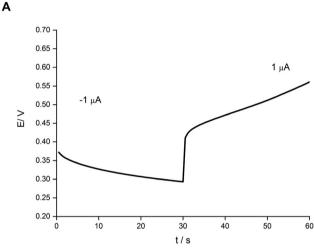
Fig. 3 (A) Nyquist plot and (B) chronopotentiometric cathodic/anodic curve ( $\pm 1\,\mu$ A) for potassium-selective ISEs.
