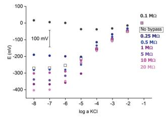
Fig. 2 Potentiometric calibration plots for  $K^+$ -selective ISEs, non-bypassed or bypassed by zinc wire and resistor  $R_{\rm b}$ . Bottom panel: experimental points were shifted to common value for  $\log a$  KCl = -1.
