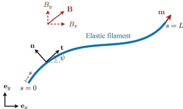
Fig. 1 Schematic diagram and notation of a model swimmer consisting of an elastic filament with a prescribed magnetic moment  $\mathbf{m}$  at one of its ends ( $s = L$ ). Here we examine the effect of shear-thinning rheology on the propulsion of the elastic swimmer under an external magnetic field  $\mathbf{B}$ .
