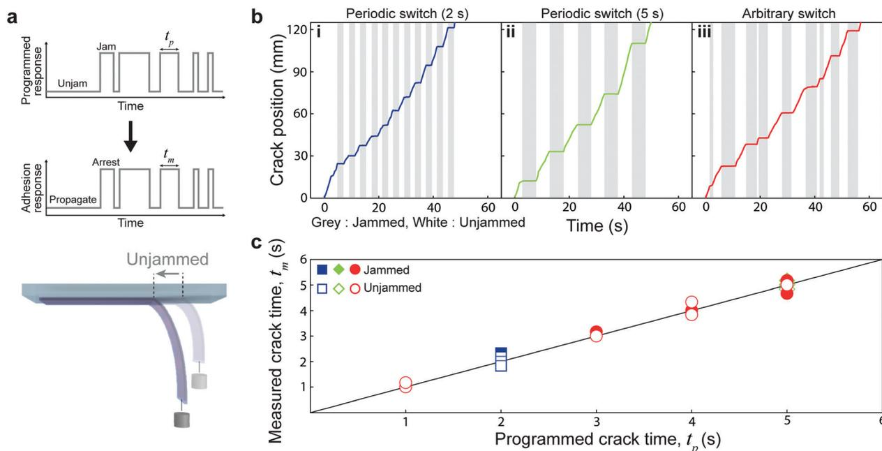
**Fig. 3** Programmability of jamming-based switchable adhesion (a) Demonstration of programmable adhesion control. (b) Crack position versus time for three different adhesion control. Cracks are programmed to get arrested in both arbitrary and periodic manners. Grey regions indicate the programmed crack behavior (Movies S2–S4, ESI†). (c) Measured crack propagation (unjammed) and arrest (jammed) show an excellent agreement with the programmed crack behavior.
