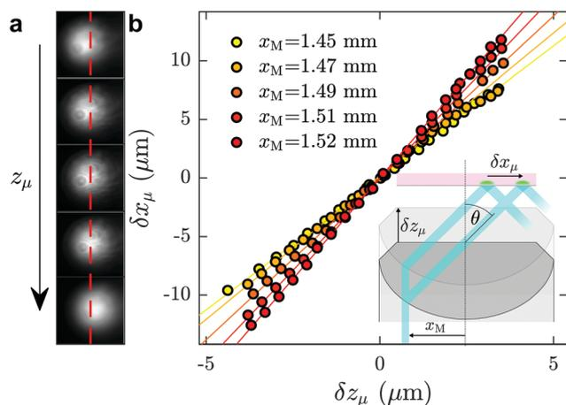
Fig. 6 Incident angle calibration. (a) Raw images of the laser beam spot for the *in situ* calibration. Successive images show the spot shifting as imposed  $z_\mu$  increases. The red dashed line represents the position of the spot when  $\delta z_\mu = 0$ . (b) Measured spot position  $\delta x_\mu$  as a function of  $\delta z_\mu$  for different values of  $x_M$ . Straight lines display linear fits of the data.
