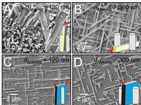
Fig. 2 TIPS-PY crystals ( $n = 1$ ) on nanopillar scaffolds ( $m = 2$ ) with nanopillar diameters and edge-to-edge spacings of (A) 240 and 120 nm and (B) 600 and 300 nm, respectively. (C and D) Perylene crystals ( $n = 2$ ) deposited on the same  $m = 2$  scaffolds, respectively. Illustrations of crystal orientations relative to the nanopillars are provided as insets. Red arrows indicate the direction(s) of fast crystallization.
