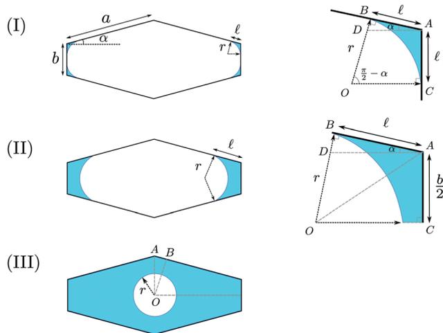
**Fig. 3** Three scenarios of the wetting liquid in the cross-section of a nearly-rectangular channel. (I) The liquid–vapor interfaces form four separated arcs in the corners. (II) The liquid–vapor interfaces form two separated arcs in the corners, with the  $b$  side is fully covered by the fluid. (III) The liquid–vapor interface is a full circle, with the perimeter of the cross-section all covered by the fluid.
