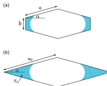
Fig. 5 Demonstration of the procedure to calculate the  $s^*$  in case (II). The meniscus position of  $s^*$  is shown in (a). For a diamond channel  $a_0 = a + b/(2 \sin \alpha)$  (b) with the saturation  $s_0^*$ , the position of the meniscus does not change in comparison with (a).
