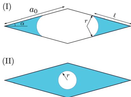
**Fig. 8** Two scenarios of the wetting fluid in the cross-section of a diamond channel. The side length of the diamond is  $a_0$  and two adjacent sides form an angle  $2\alpha$ . (I) The liquid–vapor interfaces form two separated arcs in the corners. The radius of curvature of the arc is  $r$  and the wetting length on the side is  $\ell$ . (II) The liquid–vapor interface is a full circle of the radius  $r$ .
