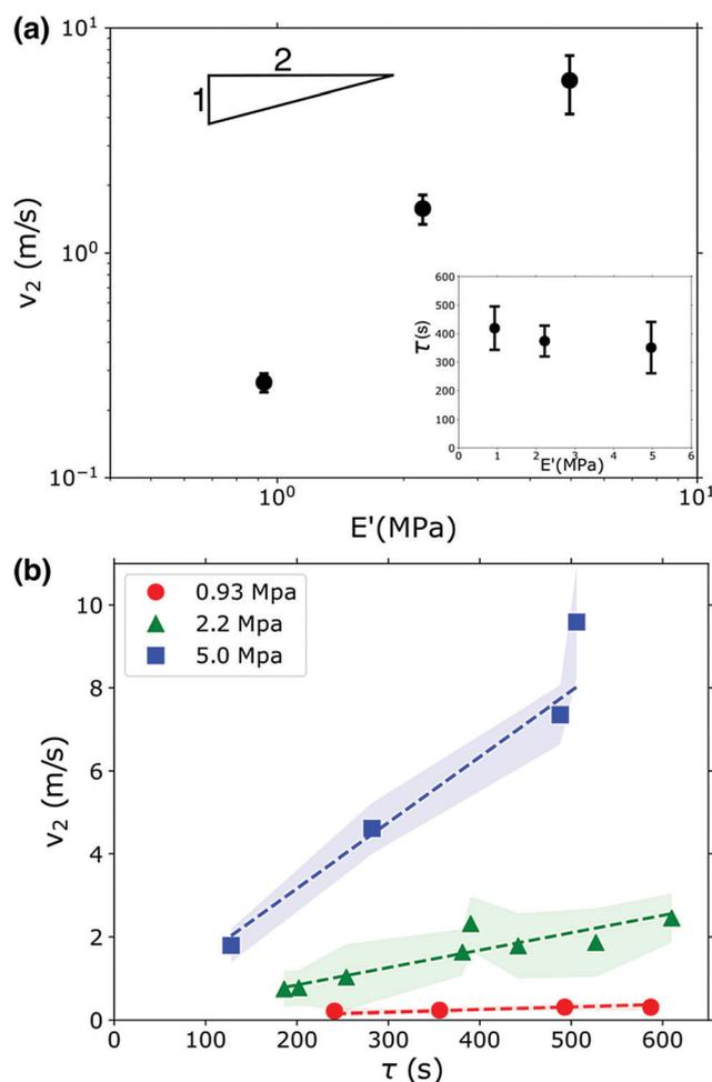
Fig. 3 (a) The mean crack velocity,  $v_2$ , increases with increasing gel modulus. However,  $v_2$  does not follow the square root scaling expected for a brittle material (square root slope is indicated by the inset triangle). The lower right inset shows that the waiting time,  $\tau$ , is uncorrelated with gel modulus. (b)  $v_2$  increases linearly with increasing fracture start time,  $\tau$ ; the fluctuations in  $v_2$  are indicated by the shaded region.
