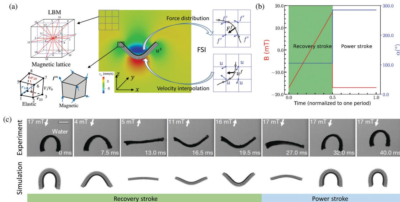
Fig. 6 Swimming of the magnetic robot. (a) Fluid–structure interaction scheme for the swimming of the magnetic robot. (b) Sequence of the applied magnetic field  $\mathbf{B}^{\text{applied}}$ ,  $\alpha$  is equal to  $360^\circ - \theta$ . (c) Comparison of the gaits of the magnetic robot in one period: from recovery stroke to power stroke. The experimental results are adapted from Hu *et al.*<sup>9</sup>
