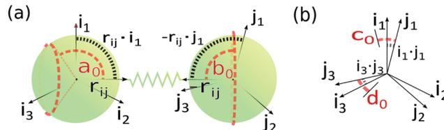
Fig. 4 Depiction of (a) bending and (b) torsional potential terms on a pair of particles  $i$  and  $j$ . The angles depicted as dot products correspond to the cosine of that angle. Equilibrium values (in red) correspond to (the cosine of) initial angle displacements derived from coordinates in the PDB file.
