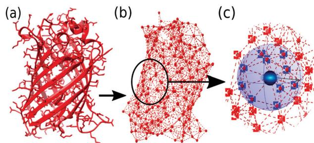
Fig. 2 Illustration of ANM using GFP protein (PDB code: 1W7S) from (a) starting PDB structure to (b) ANM representation at  $r_{\max}$  of 8 Å, (c) bonding criteria per residue: all particles within distance  $r_{\max}$  (bounds depicted by blue sphere) of center particle (black circle) are considered 'bonded' (blue squares) while those further (outside of sphere) are considered 'nonbonded' (red squares).
