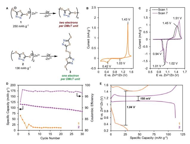
Fig. 3 (A) Oxidation of 1 and 2 to the corresponding disulfides. Solid-state CV measurements of coin cells with (B) 1 and (C) 2 as cathodes and 1 M ZnSO<sub>4</sub> aqueous electrolyte. Counter electrode: Zn. Scan rate:  $0.1 \text{ mV s}^{-1}$ . (D) Galvanostatic cycling comparison of 1 and 2 at a rate of 0.5C. (E) Typical galvanostatic charge–discharge cycling of 1 (orange), 2 (purple), and coulombic efficiency (purple triangle) of Zn-2 cells.
