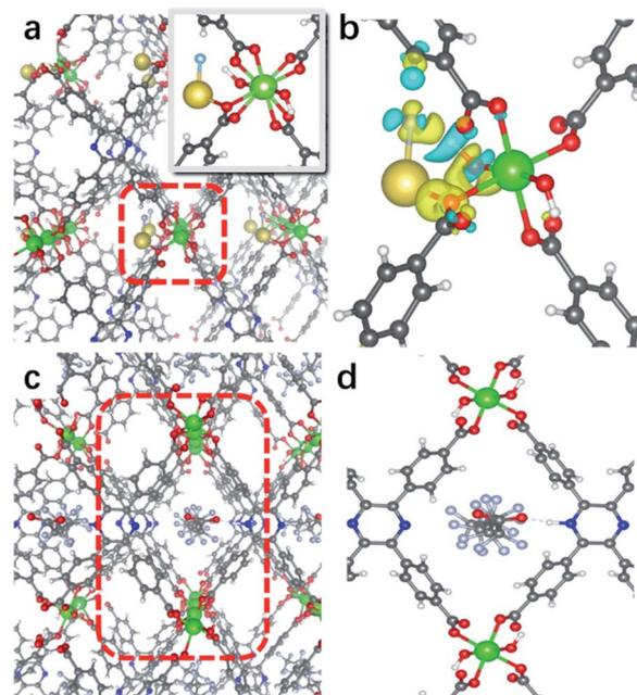
Fig. 5 (a) Optimized structure of NaF@In(tcpp), highlighting  $Na^+$  and  $F^-$  interactions. (b) Charge density rearrangement upon formation of the bond at an isovalue of  $0.002 \text{ eV } \text{\AA}^{-3}$ . (c) Binding of PFOA and In(tcpp) in PFOA@In(tcpp). (d) Configuration of PFOA@In(tcpp) (atoms are colored as follows: C grey, O red, N blue, In green, F light blue, Na yellow, H white).
