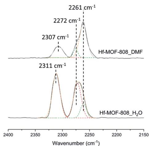
**Fig. 3** FTIR spectra of 2 mbar CD<sub>3</sub>CN adsorbed at 25 °C on Hf-MOF-808-H<sub>2</sub>O (down) and Hf-MOF-808-DMF (top). The IR bands at 2311 and 2307 cm<sup>-1</sup> are associated with CD<sub>3</sub>CN coordinated to Hf sites, and the IR bands at 2272 cm<sup>-1</sup> to OH groups in the Hf cluster. The band at 2261 cm<sup>-1</sup> is associated with physisorbed CD<sub>3</sub>CN molecules.
