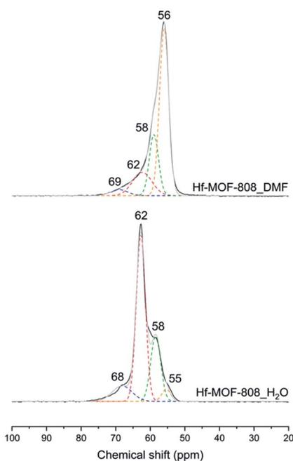
**Fig. 4** <sup>31</sup>P MAS NMR spectra of TMPO loaded on Hf-MOF-808-H<sub>2</sub>O (down) and Hf-MOF-808-DMF (top). Experimental spectra are shown in black and the sum of the deconvoluted peaks in gray.
