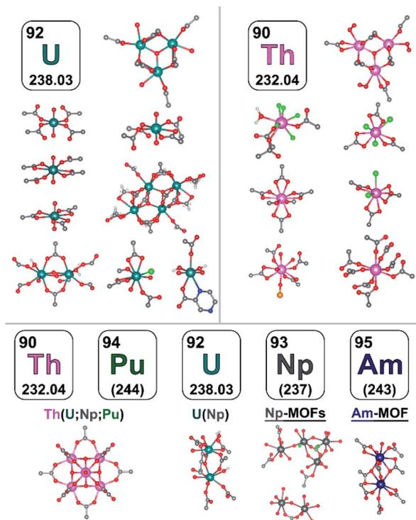
Fig. 2 Secondary building units of several examples of Th, U, Np, Pu, and Am-based MOFs. The teal, pink, dark gray, dark blue, light gray, red, blue, white, and green spheres correspond to uranium, thorium, neptunium, americium, carbon, oxygen, nitrogen, hydrogen, and halogen atoms, respectively.
