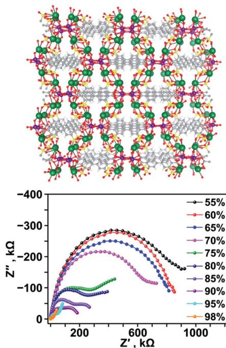
Fig. 4 (Top) X-ray crystal structure of  $K_2(UO_2)(\mu_3-O)(BPDSDC)_{0.5}(H_2O)_2$  and (bottom) Nyquist plots of  $K_2(UO_2)(\mu_3-O)(BPDSDC)_{0.5}(H_2O)_2$  collected under varied relative humidity percentages at 85 °C. The gray, white, yellow, red, purple, and green spheres represent carbon, hydrogen, sulfur, oxygen, uranium, and potassium atoms, respectively. Reproduced from ref. 97 with permission from American Chemical Society, Copyright 2020.
