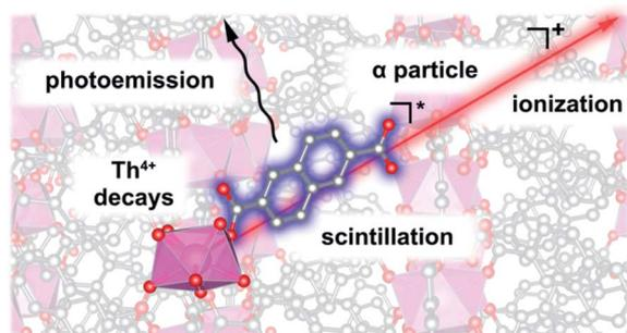
Fig. 7 Autoluminescence in Th<sub>2</sub>(NDC) occurring through emission of an alpha particle from a thorium cation, subsequent ionization of the scintillator (NDC<sup>2-</sup>), followed by core-hole recombination that leaves the system in an electronic excited state, and then visible light photoemission. Reproduced from ref. 237 with permission from American Chemical Society, Copyright 2018.
