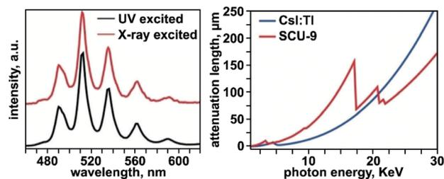
Fig. 6 (Left) Emission profile of  $\text{UO}_2(\text{HBTA})(\text{H}_2\text{O})$  (SCU-9) under UV (black) and X-ray (red) excitation. (Right) X-ray attenuation lengths for  $\text{UO}_2(\text{HBTA})(\text{H}_2\text{O})$  (red) and CsI:Tl (dark blue) in the X-ray energy region ranging from 30 eV to 30 keV. Reproduced from ref. 224 with permission from John Wiley and Sons, Copyright 2018.
