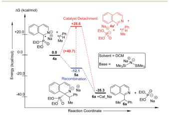
Scheme 3 Computed C–C bond formation and subsequent rearomatization energy profile.
