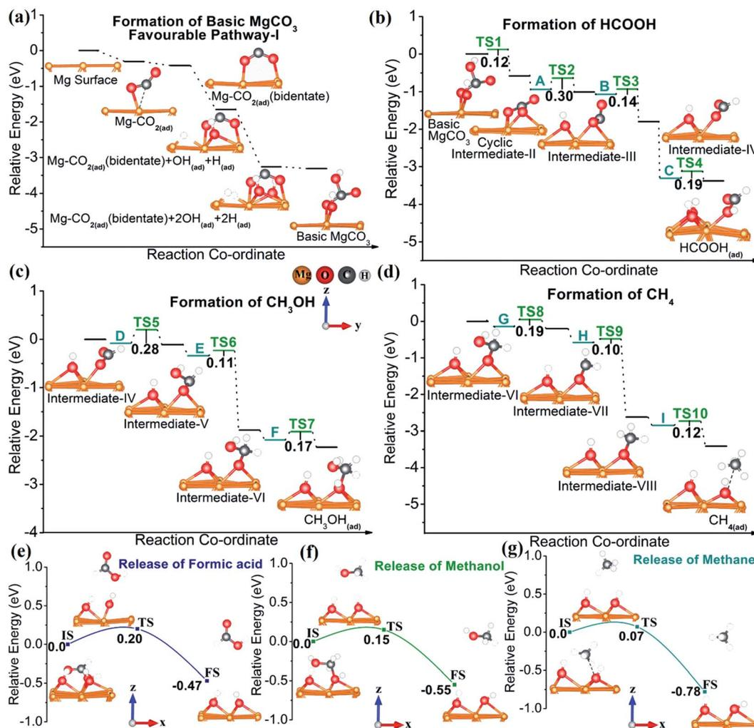
Fig. 5 Potential energy surface (PES) for CO<sub>2</sub> reduction: (a) formation of basic MgCO<sub>3</sub> via pathway-I (for the PES of pathways-II & III see Fig. S10 and S11 in the ESI<sup>†</sup>), (b) formation of formic acid, (c) formation of methanol, and (d) formation of methane; release steps of different products from the Mg NP surface during CO<sub>2</sub> reduction to (e) formic acid, (f) methanol, and (g) methane. z,y coordinates shown in (c) are the same for (a, b and d).
