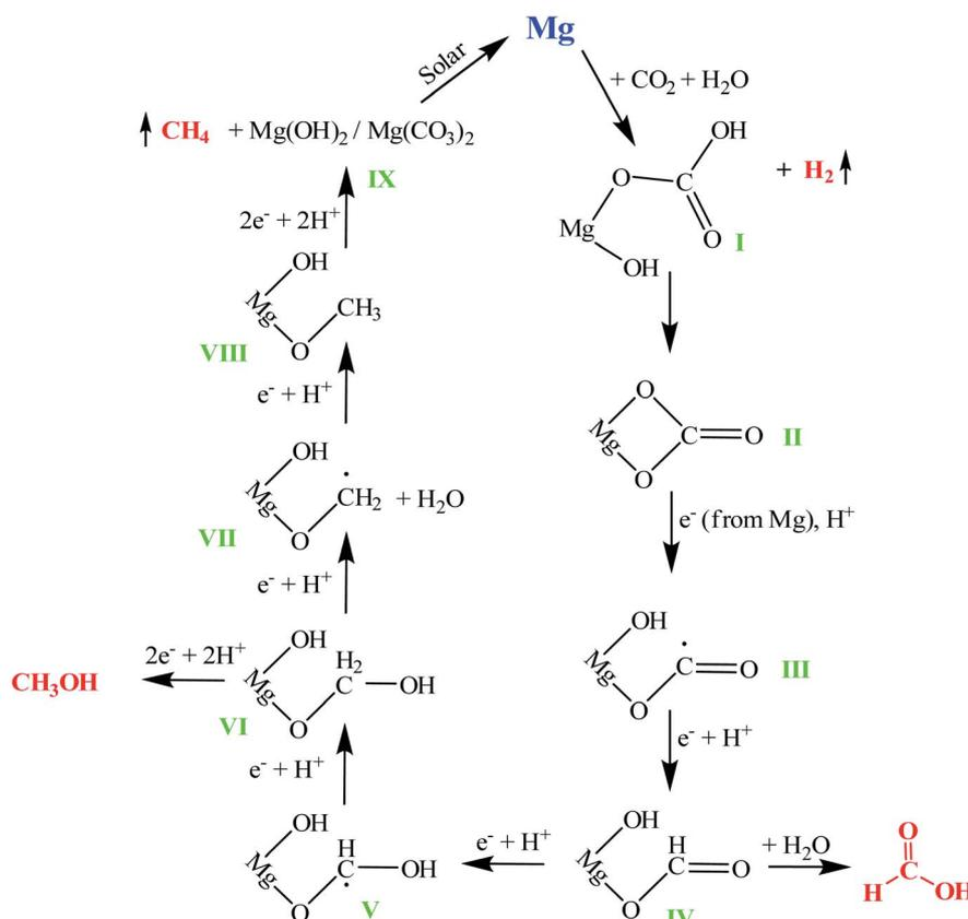
Fig. 4 Plausible reaction mechanism of  $\text{CO}_2$  conversion to methane, methanol, and formic acid by Mg using water. Mg in the scheme represents the Mg surface of nanoparticles. The upward arrow after  $\text{H}_2$  (in step I) indicates hydrogen gas release.
