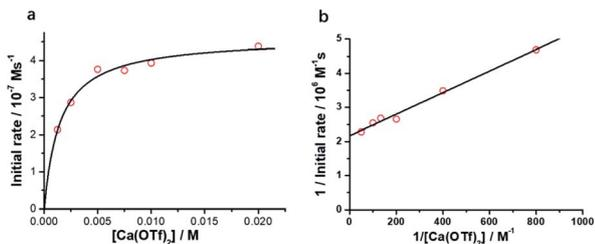
Fig. 3 Effects of  $[\text{Ca}(\text{OTf})_2]$  on cyclohexane oxidation by  $\text{RuO}_4^-$  in  $\text{CH}_3\text{CN}$ . Conditions:  $[\text{Pr}_4\text{N}][\text{RuO}_4]$  (0.01 M), cyclohexane (1.0 M) in  $\text{CH}_3\text{CN}$  at 23 °C. (a) Plot of initial rate vs.  $[\text{Ca}(\text{OTf})_2]$ . (b) Plot of  $1/\text{initial rate}$  vs.  $1/[\text{Ca}(\text{OTf})_2]$  (slope =  $(3.16 \pm 0.15) \times 10^3$ , y-intercept =  $(2.16 \pm 0.06) \times 10^6$ ,  $r = 0.988$ ).
