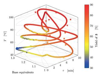
**Fig. 6** Results for run 3 of Table 1: design space where yield is represented by the color (circles: FTIR; squares: HPLC). This trajectory has no crossings.
