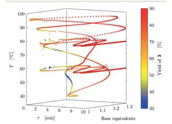
Fig. 7 Design space where yield is represented by the color (data from FTIR) where all experiments are reported. The crossings between different experiments are circled.
