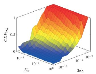
Fig. 2 CDF of deviation between dynamic and steady-state yield  $(2\sigma_{\Delta})$  as a function of  $K_{\rm T}$ .
