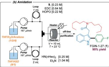
Scheme 3 Reaction setups used for preparing acid 9 and FGIN-1-27 (1).
