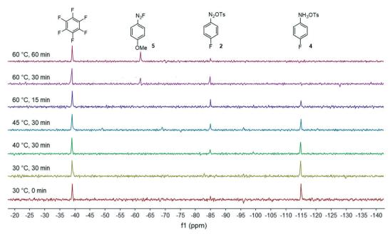
Fig. 2 Monitoring of the diazonium salt formation in MeOH by in-line <sup>19</sup>F NMR analysis at 40.88 MHz.
