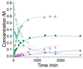
Fig. 4 Kinetic profiles for two kinetic experiments at 50 °C in methanol, with the initial concentration of maleic acid at 0.4 M and 0.8 M. At 0.4 M: • = maleic acid, — = maleic acid (ODE),  $\blacksquare$  = monoproduct, — = mono-product (ODE),  $\blacktriangle$  = di-product, — = di-product (ODE). At 0.8 M: • = maleic acid, - - = maleic acid (ODE),  $\Box$  = monoproduct, - - = monoproduct, - - = di-product (ODE).
