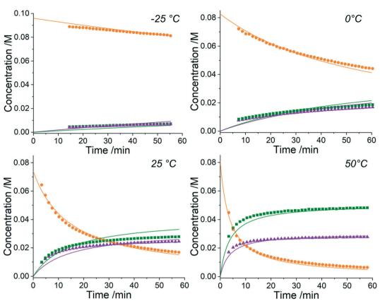
Fig. 2 Results from the four kinetic experiments (at -25 °C, 0 °C, 25 °C and 50 °C) in the S<sub>N</sub>Ar case study in CD<sub>3</sub>OD, where: • = 2,4,6-trichloropyrimidine,  $\blacksquare$  = major product,  $\triangle$  = minor product, — = 2,4,6-trichloropyrimidine (ODE), — = major product (ODE), — = minor product (ODE).
