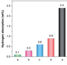
Fig. 7 Hydrogen adsorption spectra (left) and capacities (right) of (a) PCNFs, (b) 0.1 F-PCNFs, (c) Li-0.01F-PCNFs, (d) Li-0.05F-PCNFs, and (e) Li-0.1F-PCNFs composites at 0 °C under a hydrogen pressure of 10 MPa.
