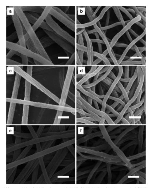
Fig. 4 SEM images of (a) porous PAN, (b) PCNFs, (c) porous PAN/PFSA, (d) 0.1F-PCNFs, (e) 0.1Li-porous PAN/PFSA, and (f) 0.1Li-F PCNFs composites. The scale bar is 500 nm.
