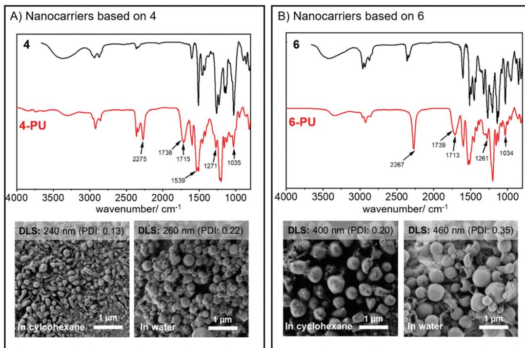
**Fig. 3** Characterization of lignin-like nanocarriers based on monomers **4** (A) and **6** (B). Top: FTIR spectra of the lignin-based monomers **4** (A) and **6** (B) before (black) and after (red) reaction with toluene diisocyanate. Bottom: Representative SEM images of the nanoparticles in cyclohexane and water, respectively; above the images, data from dynamic light scattering are summarized.
