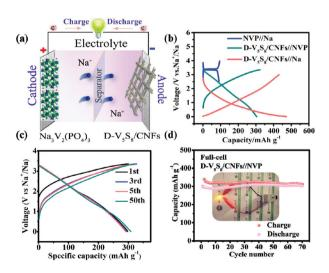
Fig. 5 The energy storage performance of a D-V $_5S_8$ /CNF full cell. (a) Working mechanism of the full cell. (b) Typical charge–discharge curves of the NVP cathode, the D-V $_5S_8$ /CNF anode and the D-V $_5S_8$ /CNFs//NVP full cell. (c) Galvanostatic charge/discharge profiles. (d) Cycling performance of the D-V $_5S_8$ /CNFs/CNFs//NVP full cell at a current density of 500 mA g $^{-1}$ . Inset of (d): an LED lightened by the flexible D-V $_5S_8$ /CNFs//NVP full battery.
