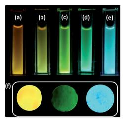
Fig. 1 C-dots2 (a) initially and after (b) 30 minutes, (c) 1 hour, (d) 1.5 hours and (e) 2 hours of sunlight irradiation. (f) Cyan, yellow and green fluorescent solid carbon dots.
