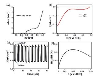
Fig. 7 (a) Tauc's plot of C-dots2 and (b) the linear sweep voltammogram of C-dots2; (c) light on–off cycle and (d) efficiency curve of C-dots2.
