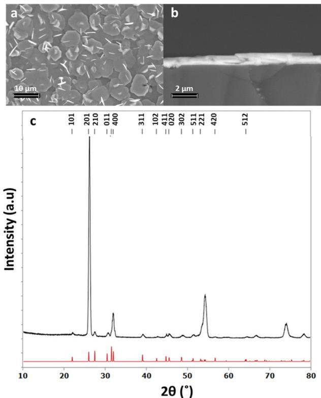
Fig. 4 Top down SEM image (a), cross sectional SEM image (b) and grazing incidence XRD pattern (c) for SnS thin film obtained by low pressure CVD using  $[\text{Sn}^{\text{n}}\text{Bu}(\text{S}^{\text{n}}\text{Bu})_2]$  (red = XRD pattern for bulk  $\text{SnS}^{48}$ ) with a thickness of around 700 nm.
