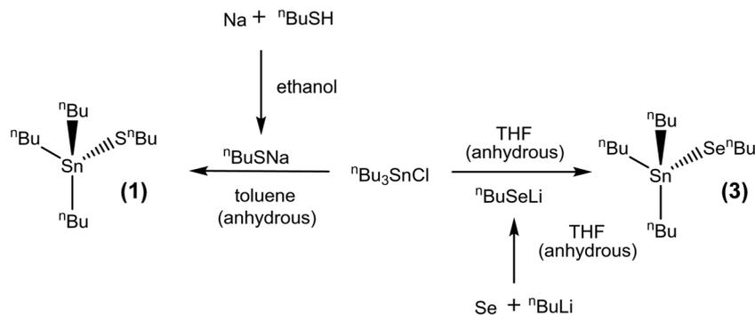
Scheme 1 Synthesis of  $[\text{Sn}^n\text{Bu}_3(\text{E}^n\text{Bu})]$  (E = S, Se) (1) and (3).
