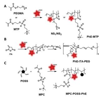
Fig. 11 Examples of polymerization using vinyl terminated AlEgens as FMs: (A) PhE-MTP developed by Ma et al. and Liu et al., (B) PhE-ITA-PEG described by Ma et al. and (C) MPC-POSS-PhE described by Huang et al.
