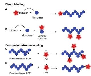
**Fig. 9** General strategies to incorporate a FM into a block copolymer backbone. Direct labeling by means of a fluorescent initiator (A) or a labeled monomer (B). Post-polymerization labeling using reactive functions on the polymer backbone (C) or at the terminal end (D). The FM is represented as a red star.
