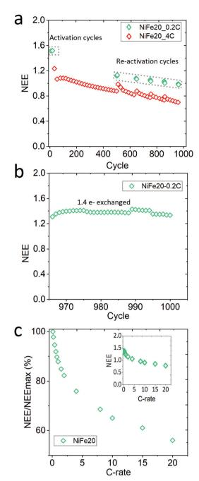
Fig. 5 Characterisation of NiFe20 stability: (a) long-term stability test, (b) after the long-term stability test the electrode is repressed and the capacity of NiFe20 goes back to 1.4e exchanged, and (c) high rate performance of the repressed electrode after the long-term stability test represented by NEE normalised by NEE at 0.1C.
