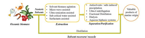
Fig. 8 General scheme for the extraction and purification of renewable chemicals/products from oceanic biomass.
