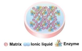
Fig. 14 Schematic presentation of an ionic liquid gel. The matrix exterior protects the enzyme and the ionic liquid supports enzyme activity.
