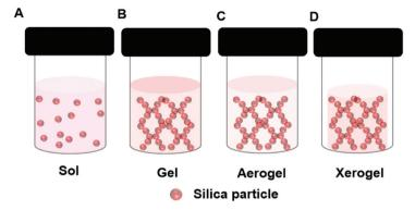
Fig. 4 Schematic presentation of different structures formed during the sol-gel formation of a silica gel depicting a (A) Sol, (B) Gel, (C) Aerogel, (D) Xerogel.
