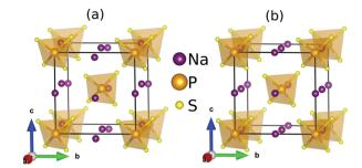
Fig. 1 The crystal structure of (a) low temperature tetragonal phase  $(P\bar{4}2_1c)$  and (b) high temperature superionic cubic  $(I\bar{4}3m)$  phase of Na<sub>3</sub>PS<sub>4</sub>.
