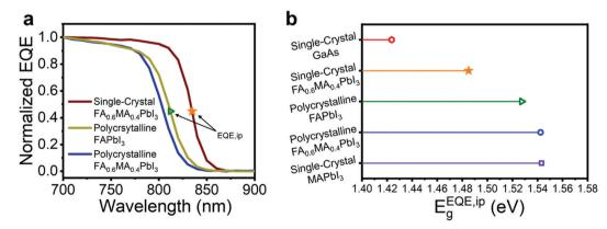
Fig. 4 (a) EQE spectra comparison between the single-crystal  $FA_{0.6}MA_{0.4}PbI_3$  device and polycrystalline  $FAPbI_3$  and  $FA_{0.6}MA_{0.4}PbI_3$  devices with the same device architecture. (b) Bandgap of select absorber materials calculated from the inflection point of the EQE spectrum. The bandgap value for GaAs was obtained from ref. 25.
