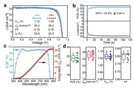
Fig. 3 (a) J-V curves of the best device under reverse (blue) and forward (red) scans. (b) Stabilized power output of the best cell at maximum power point with an applied bias of 0.94 V. (c) EQE spectrum and integrated  $J_{SC}$  of the best cell. (d) Statistical analysis of the photovoltaic parameters for 10 devices including PCE,  $V_{OC}$ ,  $J_{SC}$  and FF. Measurement was conducted under 1-sun illumination.
