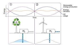
Fig. 1 Hydrogen from renewable energy is stored during periods of high renewable energy production (1) to satisfy demand during times of high energy demand and low renewable energy production (2).
