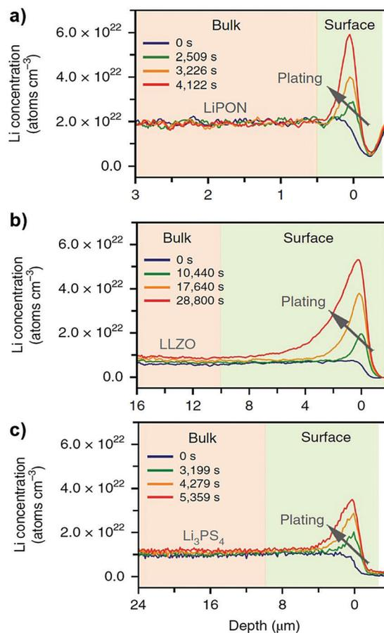
Fig. 10 Measurement of Li concentration profiles using *operando* neutron depth profiling technique across (a) LiPON (b) c-LLZO and (c) Li<sub>3</sub>PS<sub>4</sub> solid electrolytes. Reproduced from ref. 74, Copyright (2019), with permission from Springer Nature.
