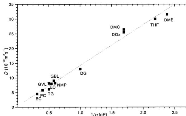
Fig. 3 The relationship between the diffusion coefficient and viscosity of 12 organic solvents. Reproduced with permission from ref. 35, Copyright (1999), American Chemical Society.
