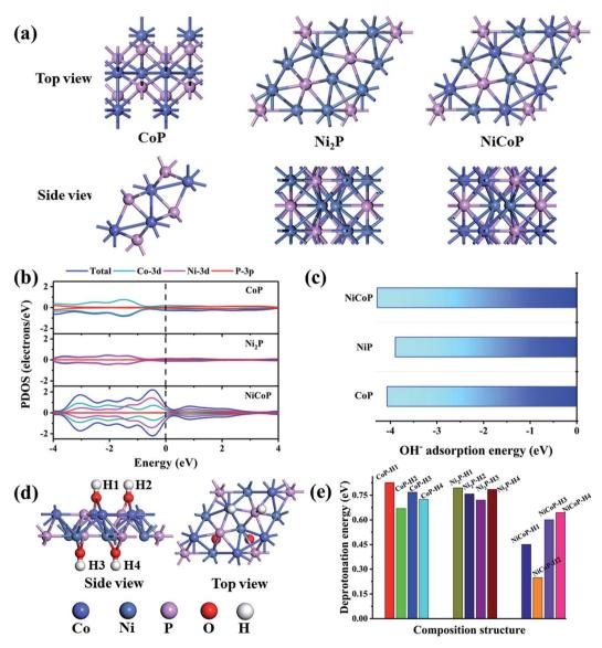
Fig. 6 (a) Top and side views for atomic structures of transition-metal phosphides: CoP,  $Ni_2P$ , and NiCoP, (b) Total and partial density of states calculated for  $Ni_2P$ , CoP and NiCoP systems, (c) adsorption energies of OH $^-$  on CoP,  $Ni_2P$ , and NiCoP systems, (d) typical representation of NiCoP $^-$ OH atomic structure, (e) the calculated deprotonation energy for the deprotonation process on CoP $^-$ OH,  $Ni_2P^-$ OH, and NiCoP $^-$ OH.
