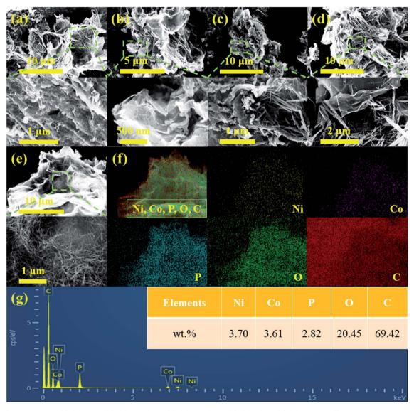
Fig. 1 The SEM images of (a) GO@Ni<sub>3</sub>Co<sub>1</sub>P, (c) GO@Ni<sub>3</sub>Co<sub>2</sub>P, (d) GO@CoP, (e) GO@NiCoP, (f) the elemental distribution sum spectra and (g) the corresponding EDS mapping of GO@NiCoP.
