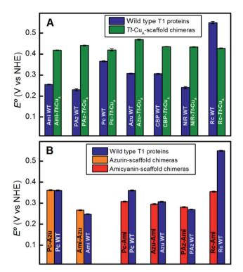
Fig. 4 (A) Reduction potentials of the Tt-Cu<sub>A</sub> chimeras compared with the corresponding native T1 sites. (B) Reduction potentials of chimeras based on the azurin and amicyanin scaffolds compared to the corresponding native sites. Except for Tt-Cu<sub>A</sub> chimeras, values are taken from literature. 5,13,45
